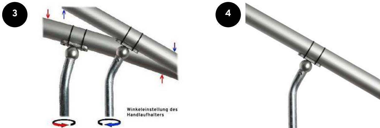
When these are aligned, screw the bracket to the railing rod using the flathead screw (12).
